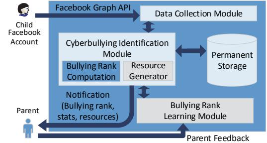
Fig. 1. BullyBlocker Architecture
